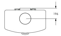
Flue Outlet To Suit 175mm (7") Flue Pipe
