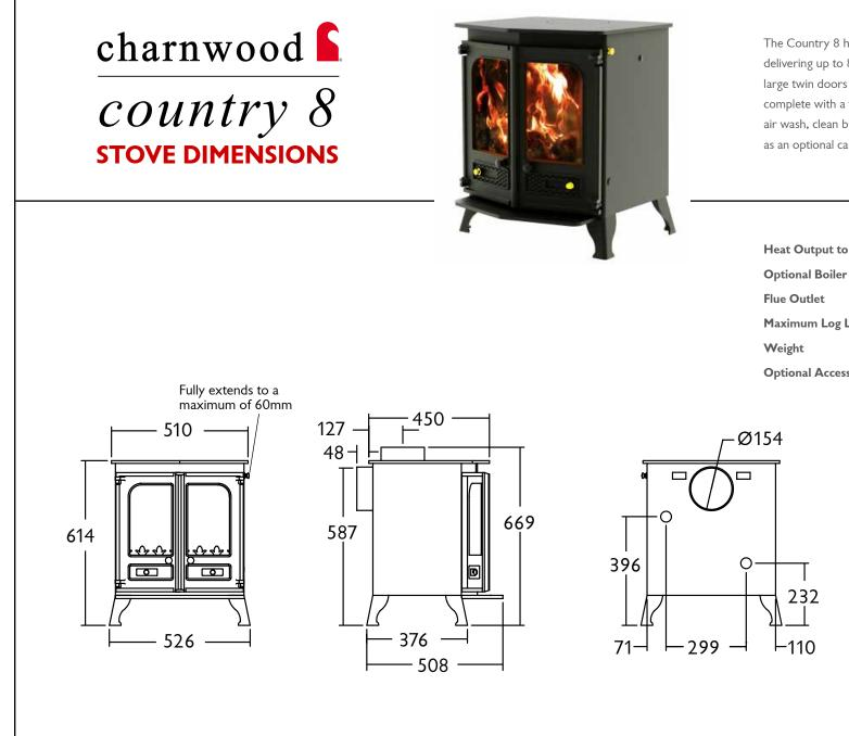
The Country 8 has always been a very popular choice of stove, delivering up to 8kW of heat to the room. Once again it has large twin doors that fold back against the stove and comes complete with a fixed front shelf. All the standard features apply: air wash, clean burn technology and brick firebox lining, as well as an optional canopy to transform its looks.
