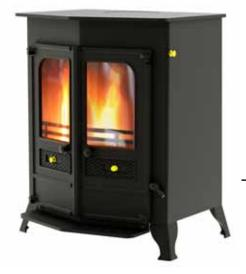
THE COUNTRY 16b Multi-fuel delivers heat suitable for heating domestic hot water plus around 10 radiators. It has a total output of 19.2kW providing 13.7kW to the water and 5.5kW to the room. Once again it is thermostatically controlled with a multi-fuel riddling grate allowing a wide range of solid fuels to be burnt. Its deep fire bed allows solid fuel to be loaded up for excellent overnight burning performance.
